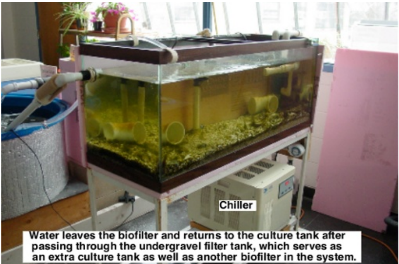
(A) Culture or Habitat Tank (B) Particle Bag Filter (C) Circulation Pump (D) Biofilter (E) Undergravel Filter Tank (F) Chiller
