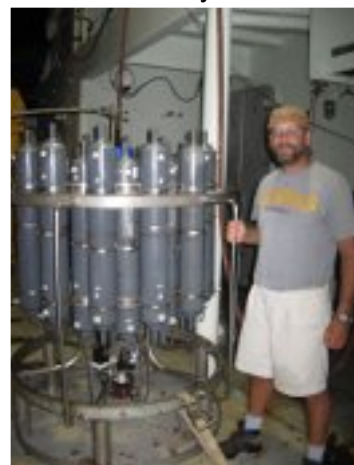
Bob on the busy deck of the R/V Knorr with the CTD tool used to measure essential physics properties of sea water.
